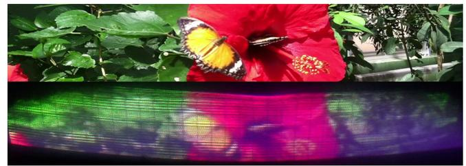
**Fig. 12.** A frame of a test color video (top) in reference to its equivalent 1-view stereogram Holographic Monitor output (bottom). See Visualization 2 for more detail.
